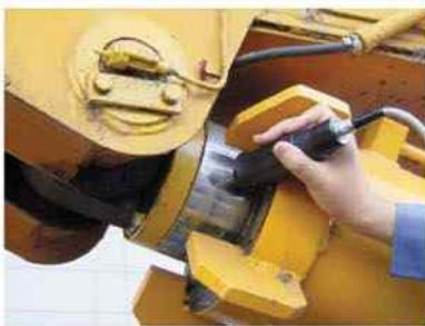
● Diagnosing wear and tear using hardness measurements
